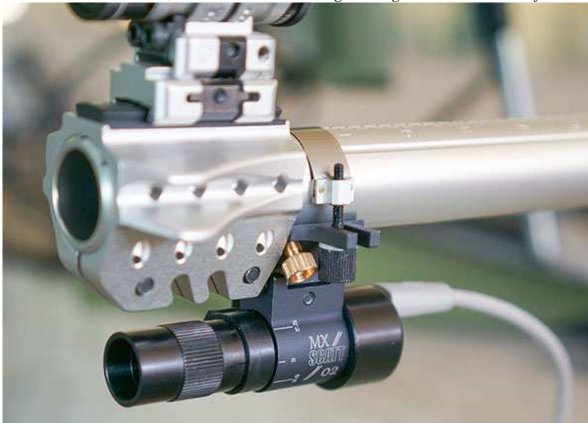
The SCATT MX-02 sensor, seen mounted on a Grünig & Elmiger Racer smallbore rifle
